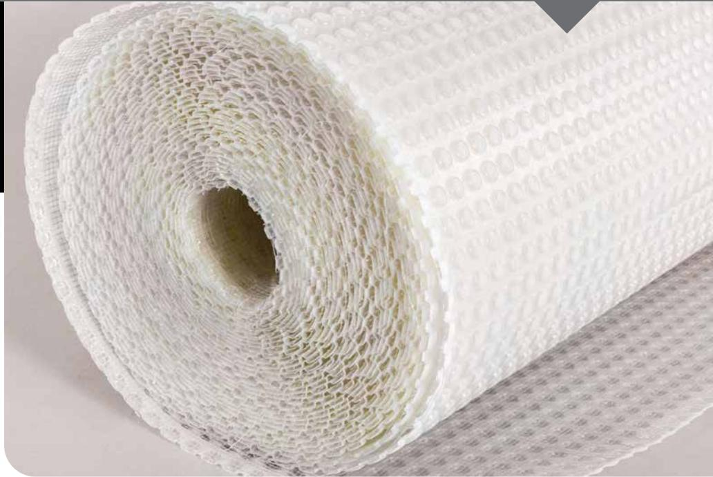
**CM3 Cavity Drain Mesh Membrane** is a 3 mm studded membrane incorporating a tough HDPE mesh lathing welded to the front face, allowing the direct application of various plaster finishes, adhesive 'dabs' and plasterboards and delivering a grade 3 environment to BS8102:2009 and NHBC Chapter 5.4.
