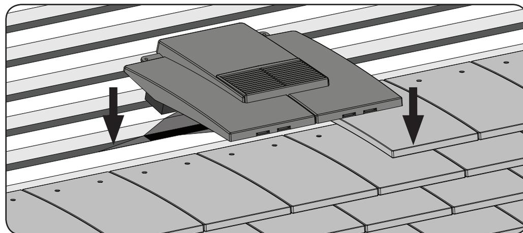
5. Slot the vent into the position. Make sure the spigot passes fully through the felt so it is accessible from the loft space. On roofs with smaller batten gauges it may be necessary to flex in the spigot clip to allow it to pass through the opening. Slide the vent left or right to align it with the adjacent tiles.
