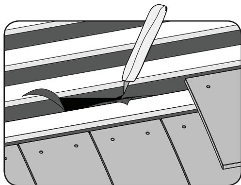
3. Cut the underlay along the diagonal X lines and fold back the triangular tabs to reveal the spigot opening.
