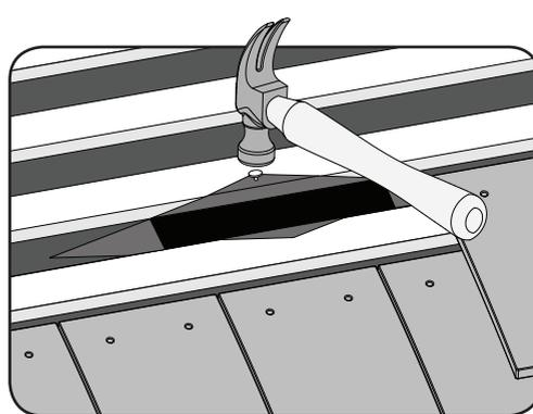
4. Fold the top tab tight up against the batten above it and secure it in position with a staple or tack.
