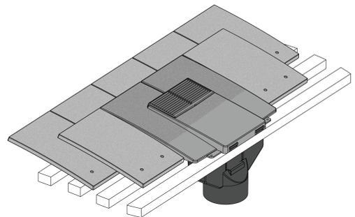
The vent outlet is designed to penetrate through the roofing underlay between the tile courses, meaning there is no need to cut or trim the battens, even when laid at the lowest batten gauge of 88mm (when using 38mm roofing battens).
