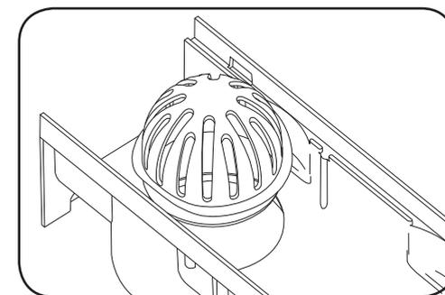
**4.** Once the channel is installed, fit the Leaf Trap into the outlet hole which has been created.
