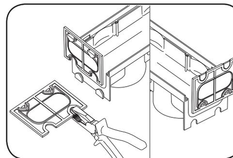
**5.** The End Cap can be fitted to either the male or female end of the channel. To fit it to the male end, first remove the thinned tabs using either a pair of pliers or heavy duty knife. Seal with a suitable silicon or polysulphide sealant.
