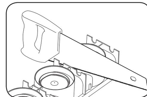
**6.** The 1m lengths of channel can easily be sawn down at several points along their length. There are saw points located on the underside of the product, next to the vertical ribs. By using these points, the interlock feature can be maintained.
