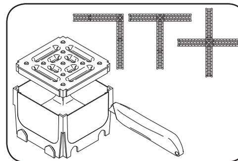
**7.** To create a junction, use a Manthorpe Junction Unit. Simply remove the correct blanked off sides with a craft knife to create either a 90° corner, T-junction or 4-way junction.
