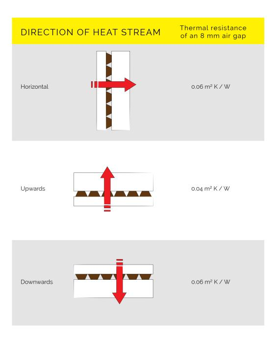
The thermal resistance values are calculated following DIN EN ISO 6946
