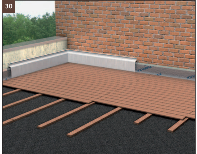
(Fig. 30) When a wooden terrace deck is to be installed on plane and firm ground, a bed of chips may be applied directly on top of the drainage sheet, after which the walkable wooden pavement may be completed.
