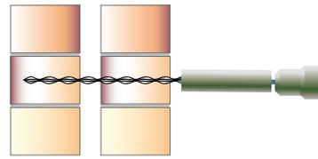
2. Insert the installation tool into an SDS rotary hammer drill, then place the tie into the installation tool.
