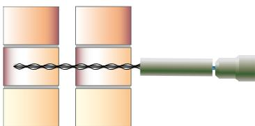
3. Drive the tie into the internal leaf to the required depth ensuring the tie is fully recessed to the external leaf below the face of the masonry.
