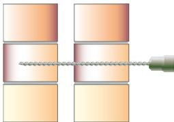
1. Drill the pilot holes through both leaves to required depth and diameter.
