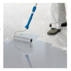
**EPOXY SEALER WATER BASED** is a two-part epoxy resin specially developed for sealing or impregnating damp or dry concrete floor surfaces that demand exceptional performances. Ideal for heavy fork trucks and to provide dust free concrete.
