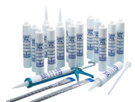
DryFix® DPC injection cream is an advanced silicone based technology used in the control of rising damp. It is a cream that is injected into holes drilled along a mortar bed using either a standard 400ml mastic applicator gun or a 5 litre applicator pump with an extension lance. Once installed, the high strength formulation spreads along the mortar bed before curing to form a damp-proof course.
