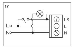
WARNING: When wiring to the PCB terminals, do not over-tighten the screws: maximum torque 0.15Nm.
