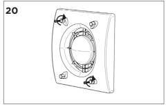
Replace the two screws removed in step 2.
