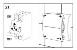
Energise the fan and check operation is correct. Then push on the front cover.
