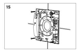
Affix the fan to the wall with the 4 screws supplied.
