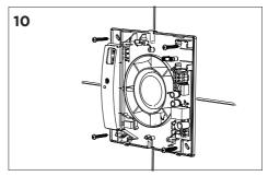
Affix the fan to the wall with the 4 screws supplied.
