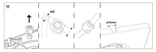
Put the cable grommet over the cable and slot into the fan. Notch the fan cover as required.
