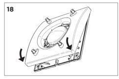
To reattach the cover, locate the 2 tabs and hinge the cover into place.
