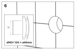
Ensure the hole or duct is the correct size for the fan.
