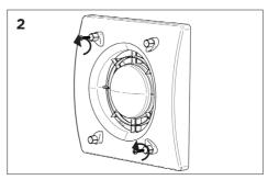
Remove the 2 screws to unsecure the front cover.
