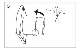
Connect the stator to the fan by locating the 2 holes and listening for the click!
