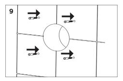
Insert the 4 supplied wall plugs. If you are mounting to other surfaces, other fixings (not supplied) may be required.
