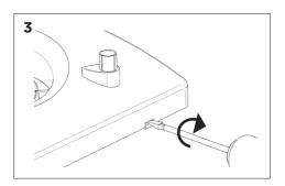
Use a flat bladed screwdriver to release the side tabs.
