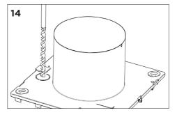
Drill/remove the rear cable knockout.
