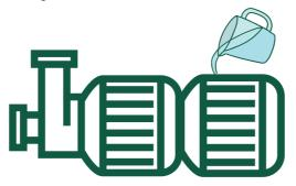
Measure accurately 4 litres of water for each 25 kg bag of NATCEM 35 into the mixer. Slowly add the NATCEM 35 whilst mixing continuously. When all the powder is added mix continuously for 5 minutes ensuring a smooth even consistency is obtained. Fluidity will only develop with sufficient mixing and will increase as mixing takes place. Do not place or pump until the desired consistency is achieved. If greater fluidity is required a total of 4.5L of water may be added.
