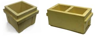
Plastic moulds are lightweight and are easy to eject using air or water pressure.
