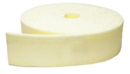
Thickness of 10mm and 12mm are available in two metre strips, or ten metre rolls. 20mm and 25mm thickness is only available in two metre strips.
