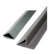
Chamfer profiles are made of impact resistant plastic and used for forming chamfer edges to columns and beams. The flanged profile is for nailing to the head of the formwork.
