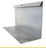
This edge trim is used as an alternative to timber shuttering on housing foundations & suspended ground floor slabs. Supplied in 1.2mm thickness as standard. 1.0, 1.6 & 2.0mm available upon request.
