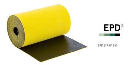
FONODAN BJ is a two layer product made of a self-adhesive high density bitumen membrane thermally bonded to a cross-linked polyethylene. FONODAN BJ acoustically works providing the acoustic mass of the tube body and removing resonant frequencies.
