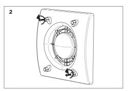
Remove the 2 screws to unsecure the front cover.
