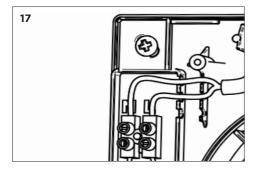
Terminate the cables as per the wiring diagram and adjust the settings for your model as shown below.
