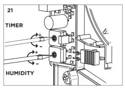
Turn the timer trimmer to adjust the run on timer from approx. 1 minute to 25 minutes. Turn the humidity trimmer to adjust the humidistat set point from between 50% to 95%. Turn the trimmer completely clockwise and the humidistat function is deactivated.
