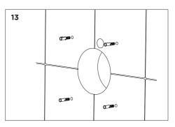
Insert the 4 supplied wall plugs. If you are mounting to other surfaces, other fixings (not supplied) may be required.
