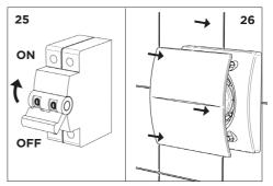
Energise the fan and check operation is correct. Then push on the front cover.
