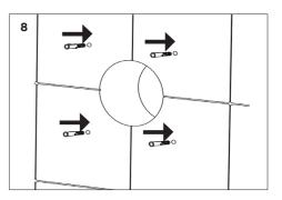
Insert the 4 supplied wall plugs. If you are mounting to other surfaces, other fixings (not supplied) may be required.
