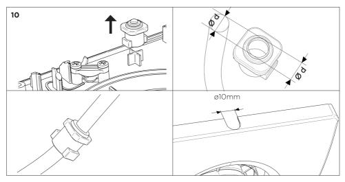
Put the cable grommet over the cable and slot into the fan. Notch the fan cover as required.
