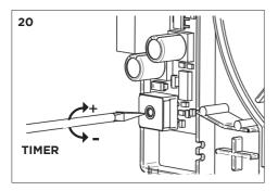
Turn the timer trimmer to adjust the run on timer from approx. 1 minute to 25 minutes.
