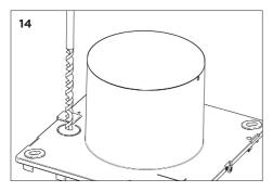
Drill/remove the rear cable knockout.
