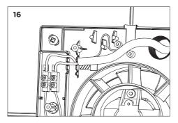
Route the cable and secure within the fan.
