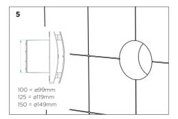
The hole in the wall should be the size noted above depending on the unit.
