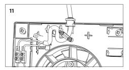
Route the cable and secure within the fan.
