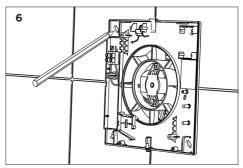
Hold the base plate up to the hole. After levelling, mark the 4 mounting holes on the wall.
