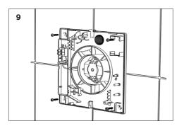
Affix the fan to the wall with the 4 screws supplied. If you are mounting to other surfaces, other fixings (not supplied) may be required.
