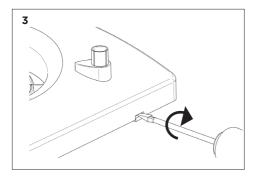
Use a flat bladed screwdriver to release the side tabs.
