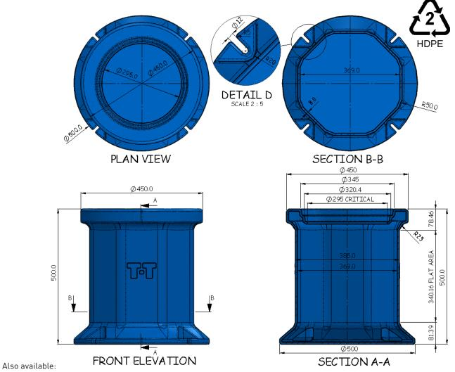
T-T Pluto Micro Extension Turret Kit, comprising additional seal and chamber riser.
